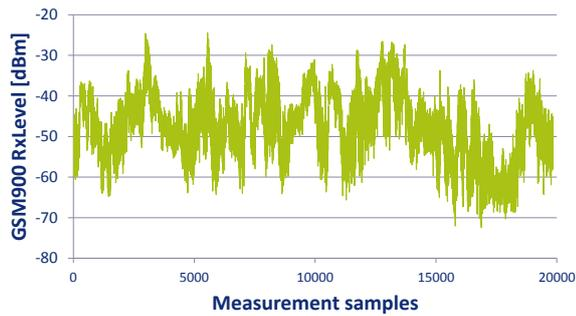
The measurements were performed with antenna located on top of the train cabin. The GSM900 levels vary mainly between -25 and -70 dBm. The probability of signal level exceeding -40 dBm was approximately 20% and exceeding -30 dBm was 1%. See detailed statistical analysis below.
