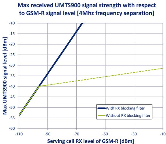
The dashed line shows our estimation for blocking performance with higher GSM-R signal levels (not verified with measurements). The blue line for filtering is applicable for frequency separation over 4 MHz. If we assume lowest possible (2.8 MHz) frequency separation for the systems, only the green line applies.
